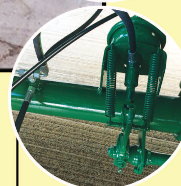
HEAVY DUTY COMMERCIAL AXLES (OPTIONAL) 420 x 180 brake shoes rated for 12 ton at 105kmh
