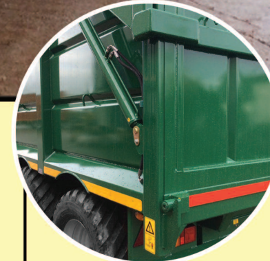
NO REAR DOOR ARMS OUT WIDER THAN THE BODY BELOW 6 FEET (HIGHER THAN A GATE POST!)
