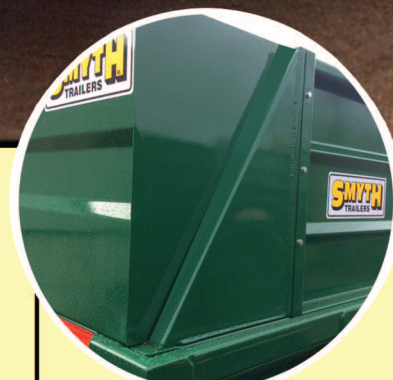
SILAGE EXTENSION INSIDE REAR PILLARS (CAN'T BE PULLED OFF BY BRANCHES)
