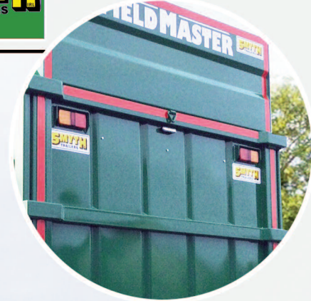
ADDITIONAL REAR DOOR LIGHTS AND STROBE LIGHT FOR EXTRA SAFETY
