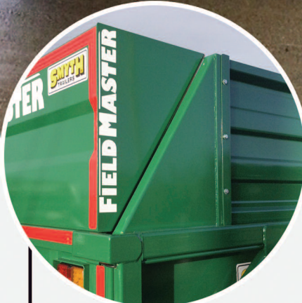
SILAGE EXTENSION INSIDE REAR PILLARS (CAN'T BE PULLED OFF BY BRANCHES)
