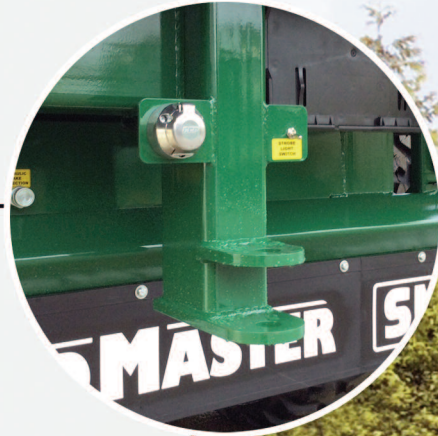
REAR HITCH C/W 7 PIN SOCKET & HYDRAULIC BRAKE CONNECTION
